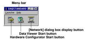
**2.** Click the start button of the desired utility, or select the desired utility from the Launcher menu.
