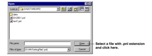
You can specify the location where the setup data file is located and open the Configurator.
