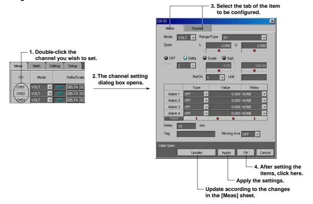
The items in the measurement channel tab can be configured for each channel. The items that are configured are the same as those configured on the spreadsheet. For details, see the page corresponding to the item.
