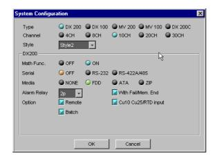
Only the system configuration in the setup data file can be checked. If the system configuration is changed and the [OK] button is clicked, a message "System Configuration is changed Input & Data are Initialized" appears. Clicking the [OK] button initializes the data.
