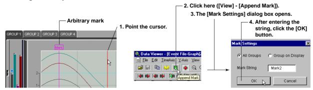
When Cursor A and Cursor B are at the same position, arbitrary marks can be placed. You can select whether to put the arbitrary marks on all groups or only on the displayed group. In addition, double-clicking a mark, that has been created using the Data Viewer, opens the [Mark] dialog box in which you can change the displayed group and the mark name.
