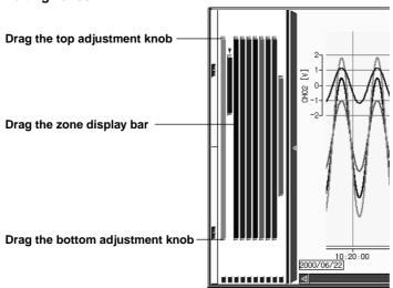
You can change the waveform display zone on the trend display screen by clicking the edit zone icon or by selecting [Y-Axis] - [Edit Zone].
