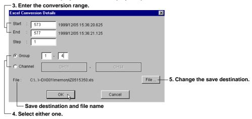
The measured data can be converted to ASCII, Lotus, and Excel formats.
