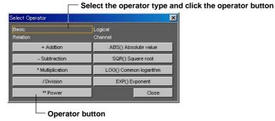
The items in the math channel tab can be configured for each channel. The items that are configured are the same as those configured on the spreadsheet. For details, see the page corresponding to the item.
